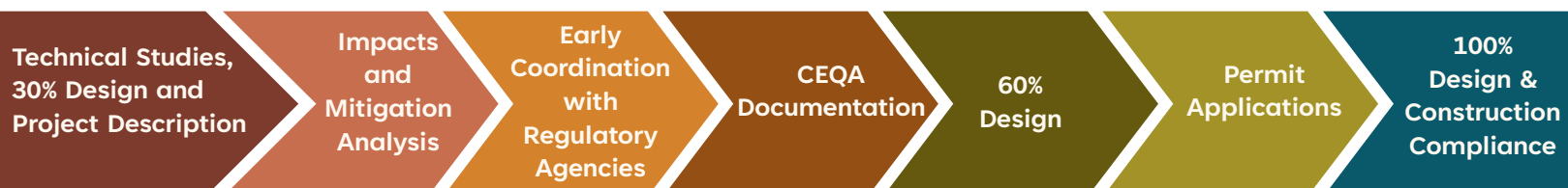
Figure 4-3: Typical Steps to Achieve Environmental Compliance Before and During Construction
