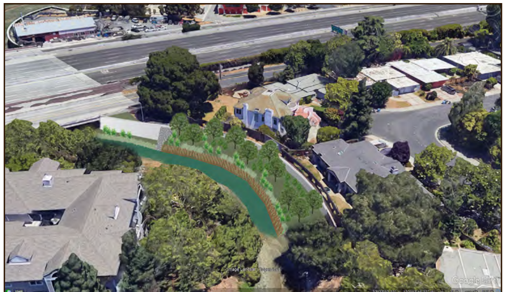
(Right) Rendering of Site 5 showing Sheet Pile wall for bridge entry and crib wall on right bank.
