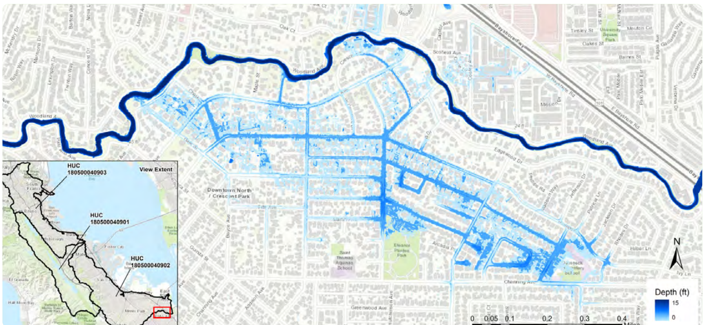
Existing 2D hydraulic model illustrating New Year's Eve 2022 runoff.
