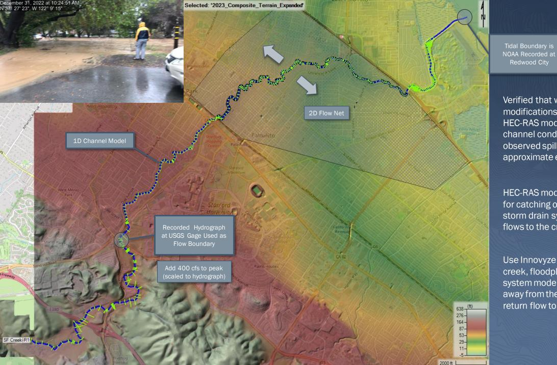
Verified that with slight modifications, the Valley Water HEC-RAS model reflects observed channel conditions and replicates observed spill locations and approximate extents.
