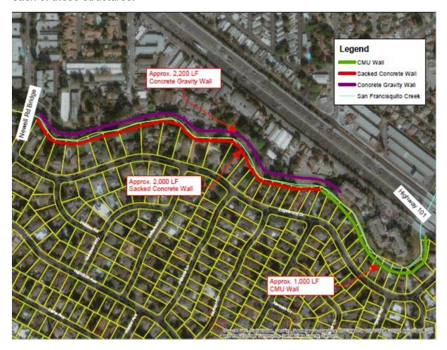
Repair of these structures has been ruled out due to condition and structural concerns. These structures and their replacement(s) fall within the general scope of the existing EIR, but the details of the construction must be addressed in a Supplemental EIR.
